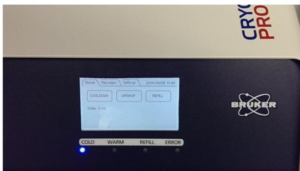
1 Front panel of the Prodigy cryocontroller
